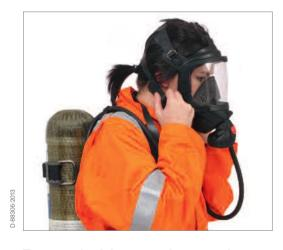
Removal of facemask, resetting LDV once face seal is broken. Close valve and vent system by
