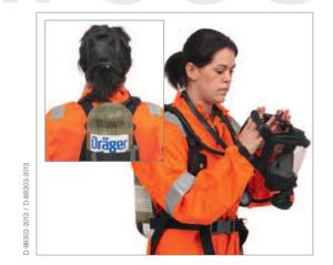
Unhook facemask from button. spread head harness and place over head with centre plate to the back. Place chin in facemask chin cup, tighten lower straps first then upper straps (holding breath). Tighten centre strap if necessary.
